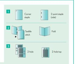
FS-527 / FS-529 Finisher Stapling Functions ► Up to 50 sheets side stapling, FS-529 corner stapling performed concurrently.
